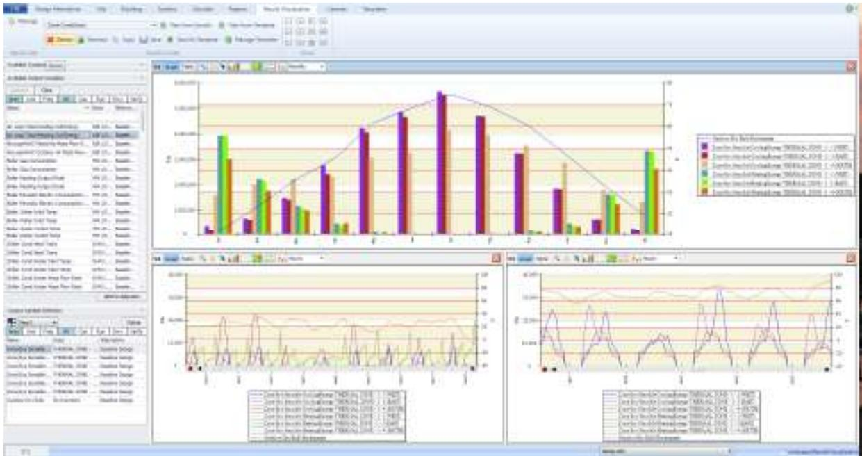
Image - Zone Conditions Results Screen Template for the sample file (ASHRAE-7\_VAV with Reheat), Simulation Configuration 2.
